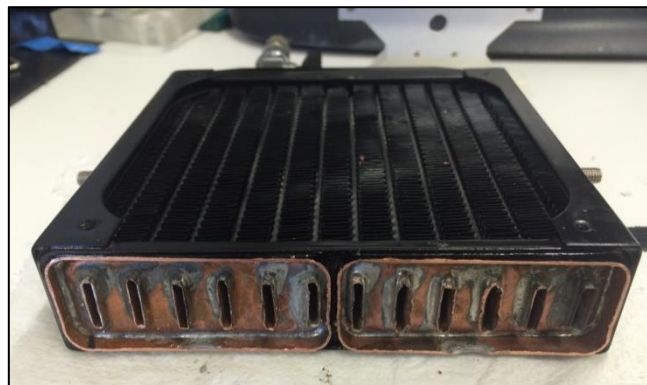
Figure 4.11 - Condenser component after band saw machine cut.
