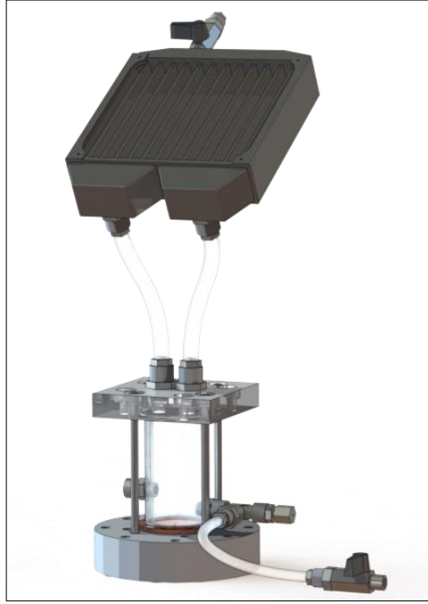
Figure 4.5 - Final design for prototype with horizontal oriented hot surface (CAD model - SolidWorks).
